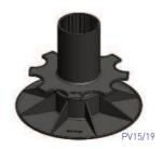
The Caro Pedestal Bases are available in four heights which, when the relevant Support Plate is chosen (for Decking, Paving and Gridded areas), will give a huge amount of choice for height variances (see pages 3 & 4). The large and easy to access threaded "wheel" adjuster gives infinite height tuning, so as to achieve the perfect flat surface.
